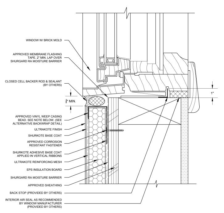
NOTE: MAINTAIN 1 SPACE BETWEEN BEVELED INSULATION AND WEEP CASING BEAD.
